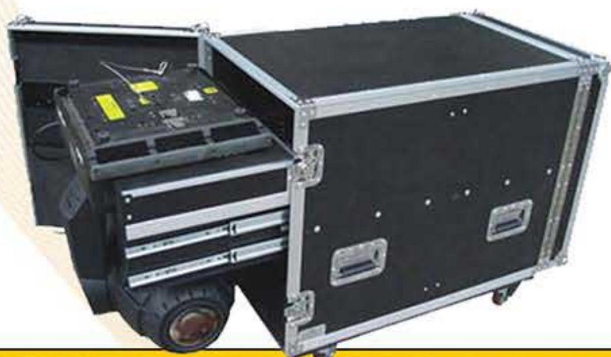
PLOK-CASE-MH Case for moving head 9mm (.35") plywood construction with laminated plastic covering 30mm (1.18") × 30mm (1.18") aluminum extrusion Heavy duty corners, heavy duty T Brackets Medium butterfly latches, medium recessed handles 4" casters (2+2 with brakes)
